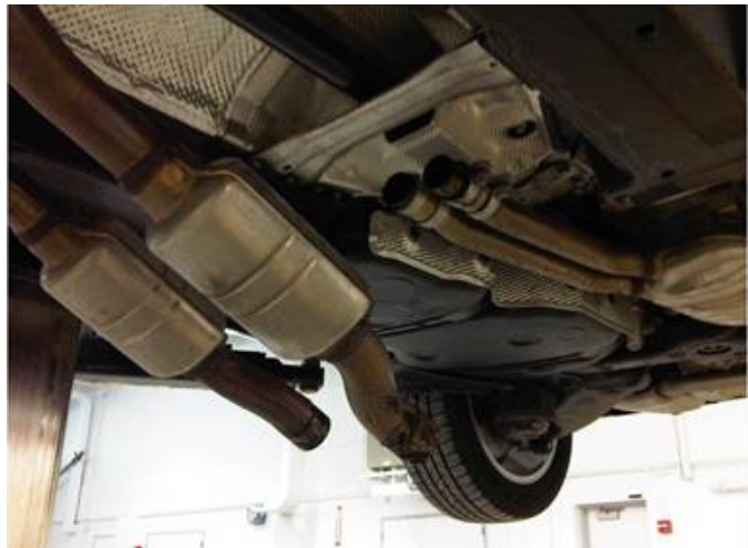
Figure 7. Lowered catalytic converter pipes
