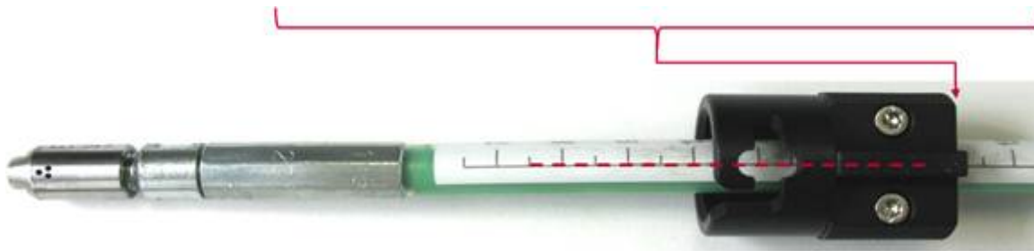
Figure 15: Arrow indicating how the back side of the adaptor must align with the scale. Red dotted line indicating how the longitudinal slot must align with the black line on the scale.
