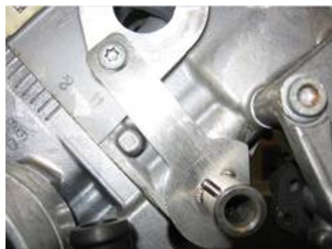
Figure 14. Engine adaptor on bank two.
