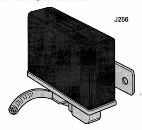
Convertible Top Control Module - J256 - is located behind the right side of the rear seatback. It oversees the entire opening and closing sequence. See page 19 for complete details.
