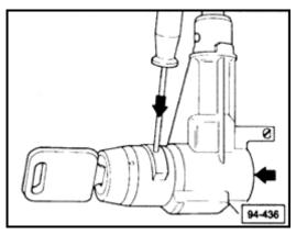
Using a punch or similar tool, press down retaining spring through hole (upper arrow), and pull lock cylinder out from housing (lower arrow).
