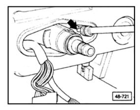
Remove steering lock housing mounting screw (Torx ® T-30) (arrow) from steering column tube.
