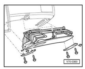
Tightening torque: 5 Nm (44 in. lb)
