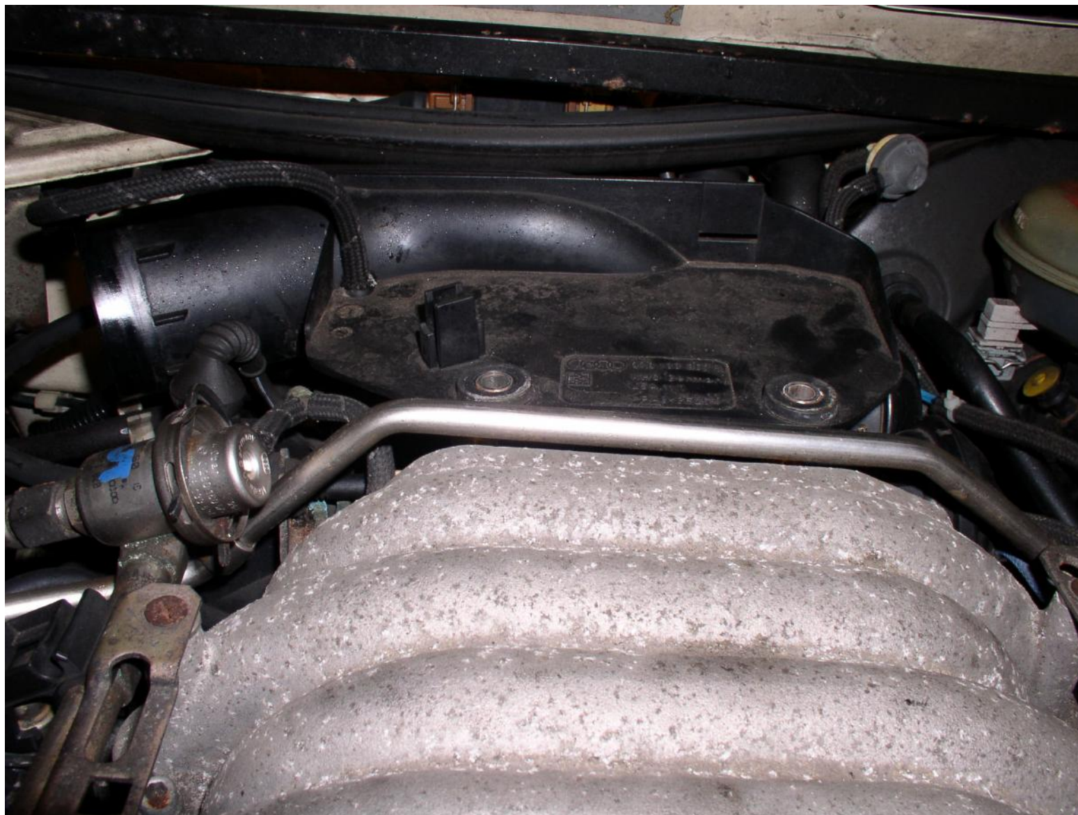
Close-up of the plenum top.
