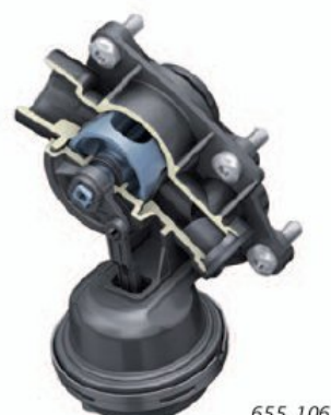
Shut-off valve closed
