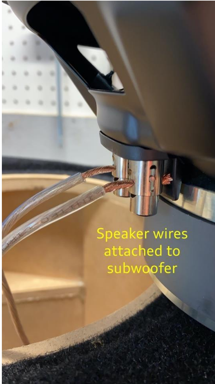
Figure 8: Speaker wires attached to subwoofer.
