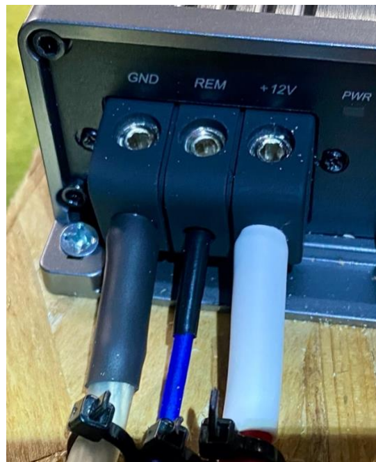
Figure 17: Example of bad power wiring at amp.
