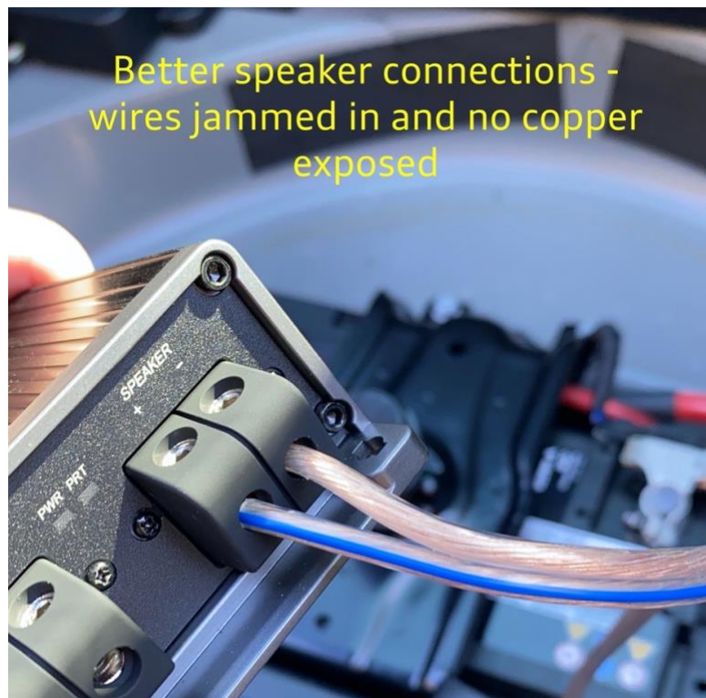
Figure 15: Better Speaker Wiring
