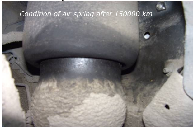
Condition of air spring after 15000 km
