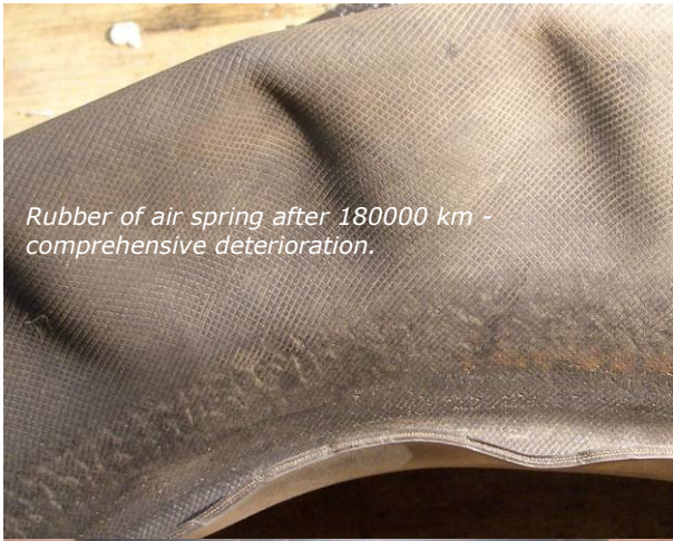
Rubber issue after 150000 km. See inner rubber surface quality
