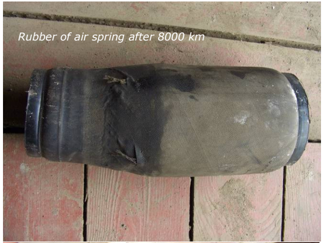
Rubber issue after 8000 km. See inner rubber surface quality
