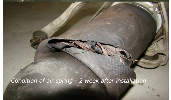
Condition of air spring - 2 week after installation. Both pictures show absence of mud which significant for old one – air spring is new.
