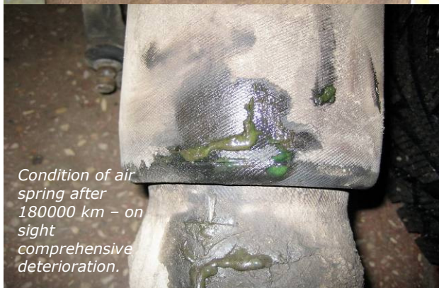
Condition of air spring after 180000 km – working surface has a lot of friction mud but no blowout.
