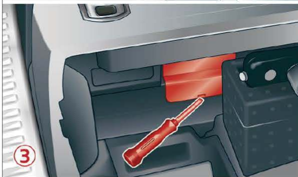
Fig. 180 Front passenger footwell: cover and clamp, left side of luggage compartment: cover
