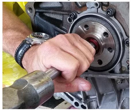
After the bushing has moved out by about  $\frac{1}{2}$  inch, remove the tool and repack the cavity with more grease:
