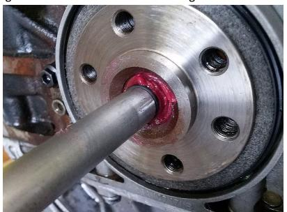
Using a large hammer, drive the tool into the bushing - Several firm hits will be required on an original bushing -
