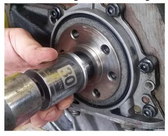
The new pilot bearing is factory filled with grease. Make sure the pilot shaft is smooth and clean before installing the transmission.
