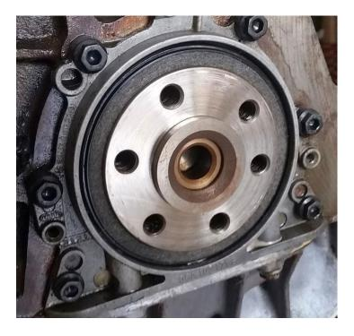
Fill the bushing cavity completely with grease. Bleed any air pockets out of the grease. Air will create a spongy feel when driving the tool in.
