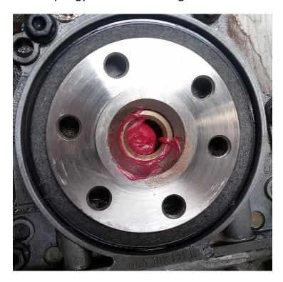
Fill the bushing all the way to the outer surface:
