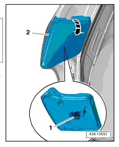
Position screwdriver -2- on opening and lever off inner cap -1- in direction of -arrow-.
