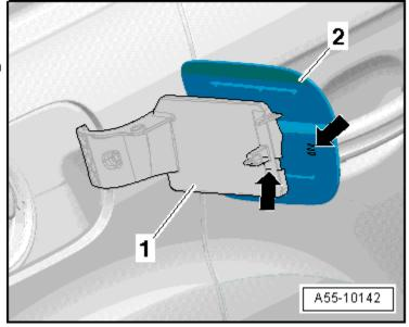
Release tank flap unit at marked locations arrows-.
