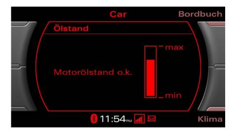
The oil level and oil temperature sender (PLUS = Packaged Ultrasonic Level Sensor) sends signals (PWM = Pulse Width Modulation) to the engine control unit relating to engine oil temperature and oil level; the oil level is displayed as mm above the mounting surface.
