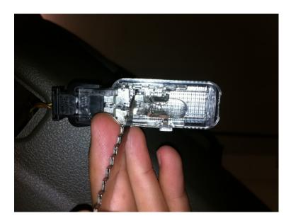
I then went on to the Visor lights. They are the same type of housing as the door puddle lights. The clip was on the left side. Just wedge a tool in there and pry it off.
