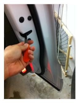
Then...you take your flat tool and pry open the light housing. You can see which end has the clip by looking at the lens and seeing one end have a little notch.
