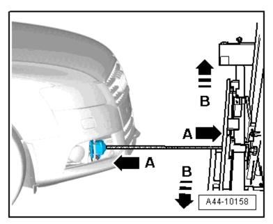
Attach front wheel alignment sensors -1to -VAS 6430-.
