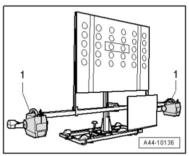
Position ACC setting device -VAS 6430so that distance -A- between sensor lens and surface of reflector is 120 cm ± 5 cm.
