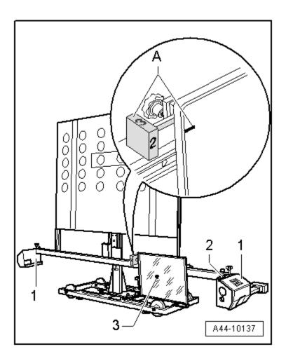
By moving it sideways -arrows B-, set -VAS 6430- so that laser beam coincides with centre of sensor lens in the horizontal plane.
