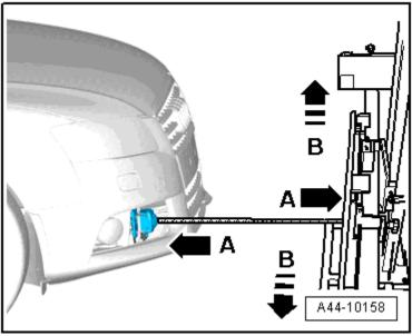
Use adjusting screws -1-, -2- and -3- to bring spirit levels -A- and -B- on -VAS 6430- into horizontal position.
