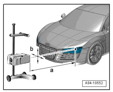
Dip setting -arrow- is marked on top edge of headlight -1- in "%".
