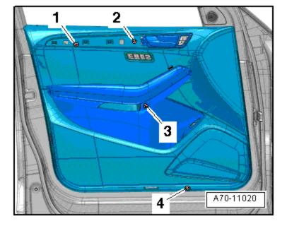
Starting in bottom rear corner, use removal pliers -3392- to unclip door trim from door.
