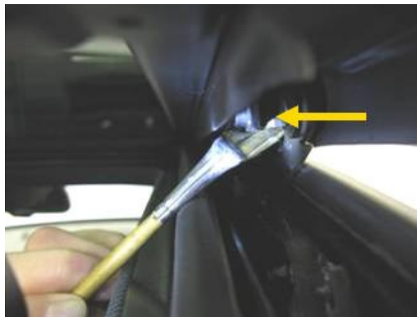
Figure 7. Locking pin for sunroof panel 1, viewed with panel 1 in a tilted position.
