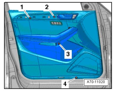
Starting in bottom rear corner, use removal pliers -3392- to unclip door trim from door.
