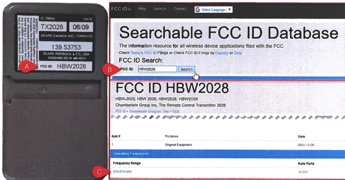
Figure 1. Checking the operating frequency.
