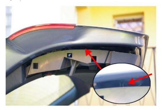
5th Connect the cable from the module to the vehicle Trunk lighting. You can do the attached Quick connectors or use the cable and then solder the Strip.
