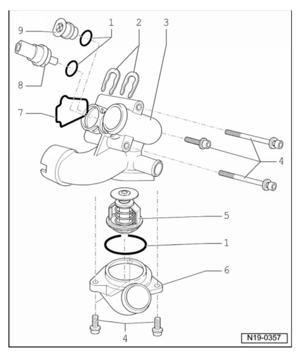
Item 8 G62 - Engine coolant temperature (ECT) sensor
