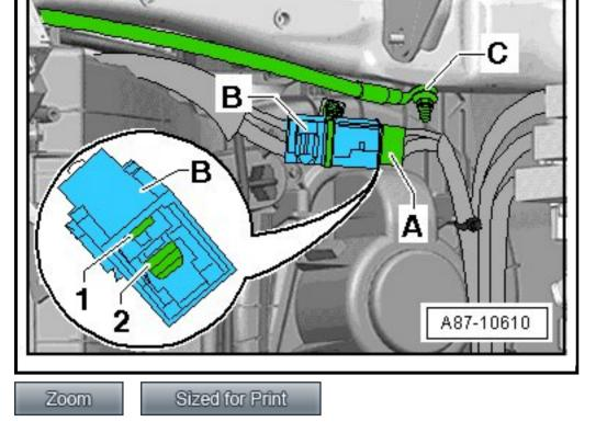
• Measure the resistance between the contact 1 inside the connector - **B** - and the ground point - **C** - on the instrument panel cross-member (for example, with the Vehicle Diagnosis, Testing and Information System (VAS 5051 A) )
