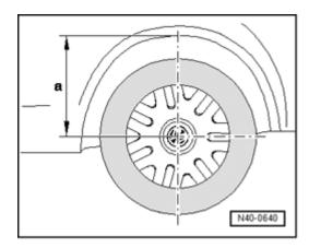
Ride height - a - is measured vertically from the fender or lower edge of the quarter panel to center of wheel.
