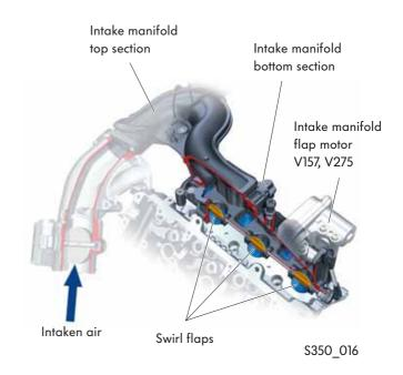
The swirl flaps are moved by the intake manifold flap motor via a push rod. To do this, the positioning motor is actuated by the engine control unit. An integrated sensor serves to feed back the current position of the swirl flaps.
