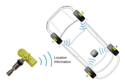
Generation II Sensors from ORO-TEK are the first aftermarket OEM replacement to offer compatibility with Wireless Auto Location systems. At the cutting edge of TPMS technology, W.A.L. systems allow for replacement sensors to be learned automatically by and interact with a single, central receiving antenna in the vehicle.
