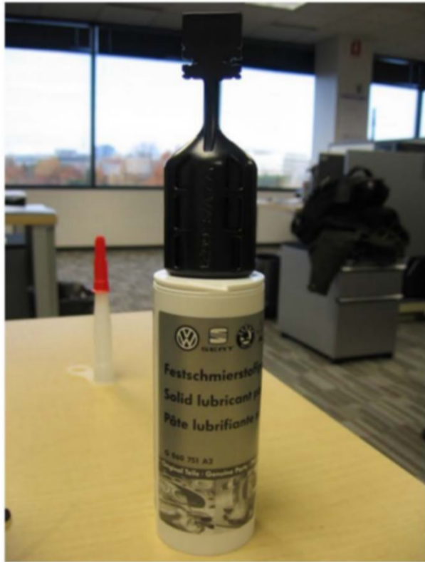
Figure 24. Lubricant with VAS 6621 installed.
