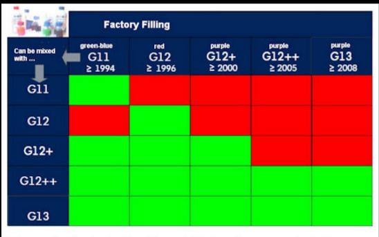
Figure 2. The table identifies which Service coolants (left) can be added to the Factory Filled coolant (top).
