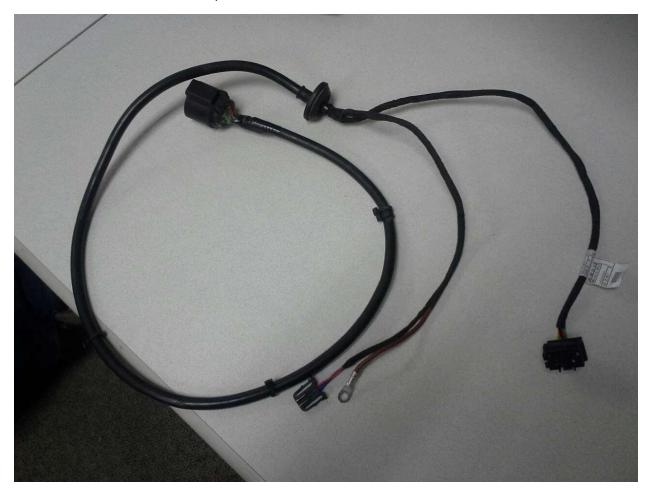
69 inches long, 45 inches to the soft plug from the 7 pin connector. At the Y one side is 19 inches with the ground strap split off with a 5 inch length at 12 inches. The control side is 24 inches after the plug.
