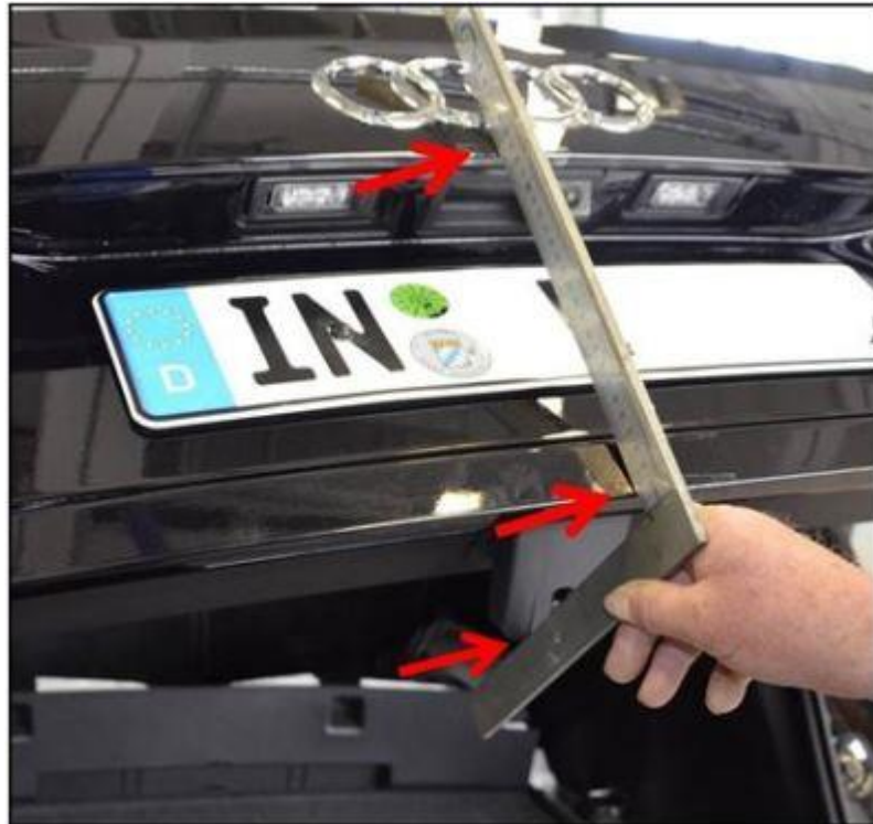
Figure 13. Checking the Rear Lid Latch geometry.
