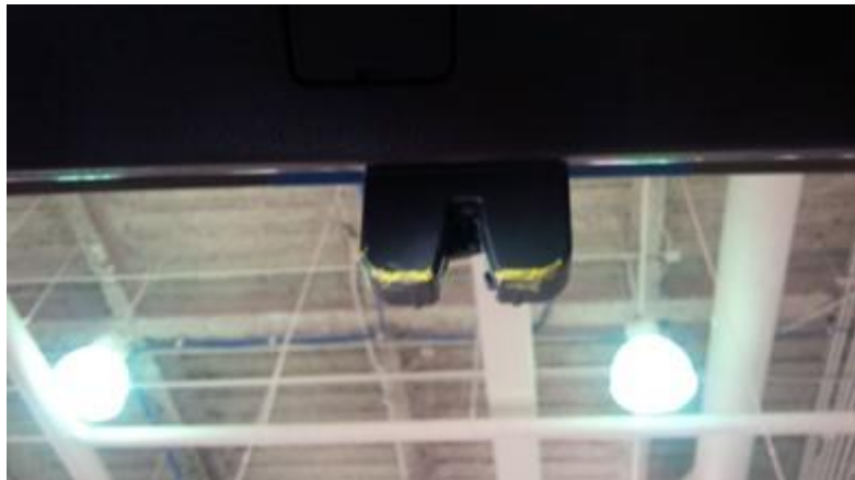
Figure 10. Tire grease pencil applied to the leading edge of the Rear Lid Latch V53.
