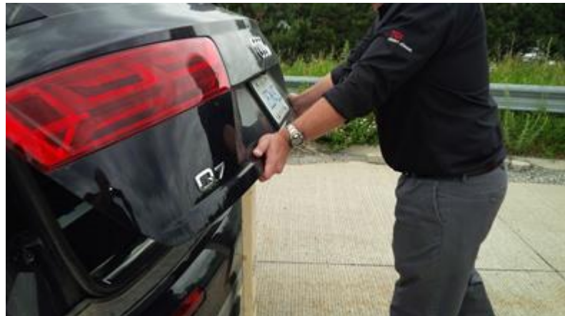
Figure 17. Applying downward pressure to rear lid to adjust latch angle.
