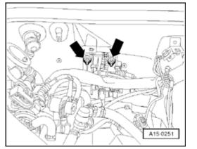
Removing oil seal at Hall sensor (left cylinder head)
