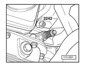
Screw clamping bolt 3242 for crankshaft into sealing plug hole and tighten.
