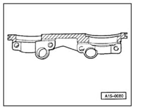
Apply a thin coating of sealant 454 300 A2 to shaded areas on double bearing cap (see illustration), install bearing cap and tighten bolts to 10 Nm.
