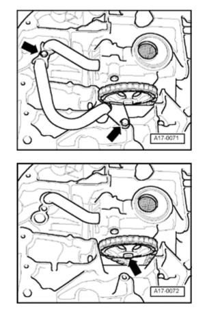
Unbolt brackets for oil supply lines -arrows- and pull front (longer) oil supply line away downward.
