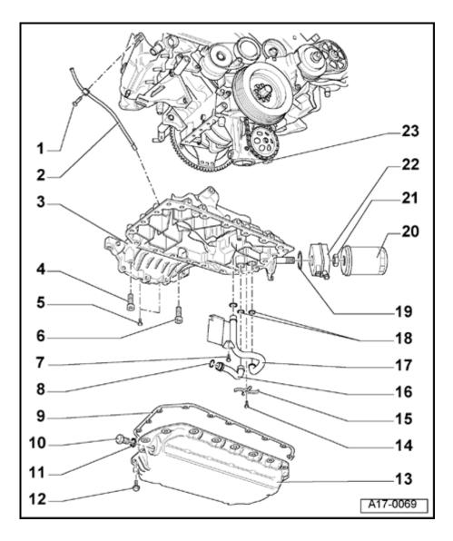
Oil pump, oil pan, oil filter and oil cooler, removing and installing
