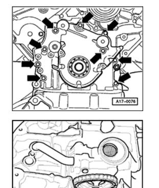
Unbolt front sealing flange and take off gasket for front sealing flange M6 bolts: 10 Nm M8 collar bolt: 30 Nm
