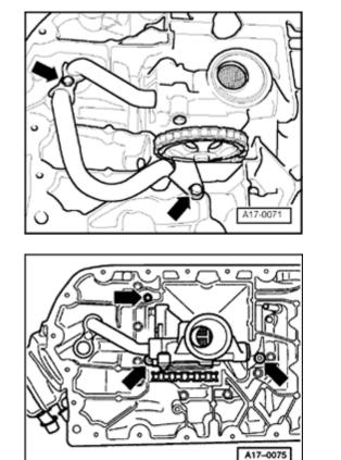
Unbolt two oil supply lines, and pull longer of two lines downward to disconnect from upper section of oil pan.
