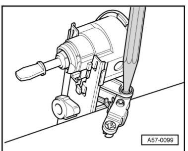
Correct Installation Position Of Spring
