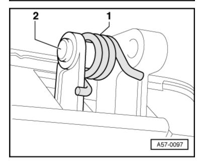
Installing Locking Pins
