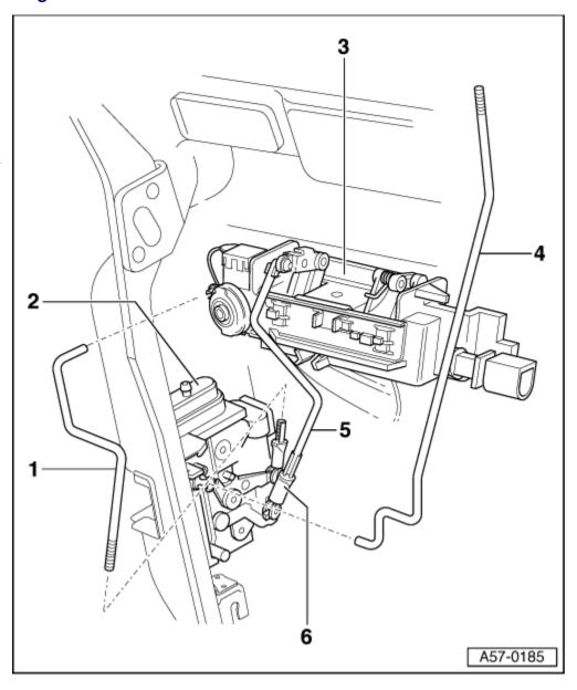
Removing and Installing Securing Rod for Lock Cylinder
