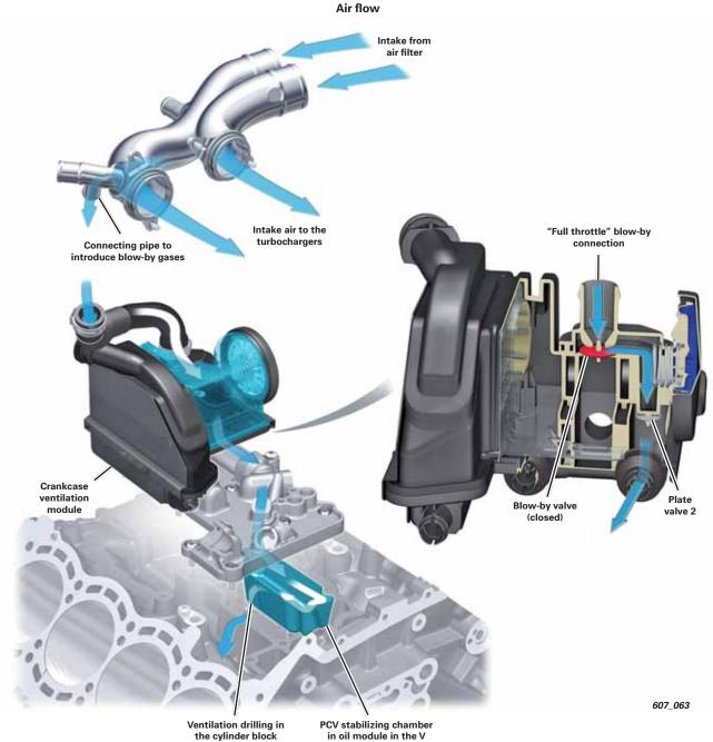
PCV stabilizing chamber in oil module in the V
