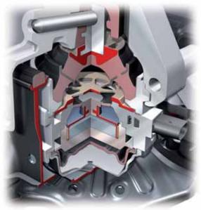
If oscillations encounter each other at the right time, the disturbing oscillations are eliminated.
