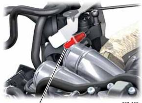
Engine Cover Temperature Sensor G765 607\_113a
