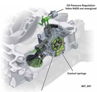
Adjustment ring at maximum delivery position
