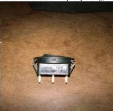
I drilled a ¾ "hole in the Rear Hatch Panel and pushed the Toggle switch securely into the panel.
