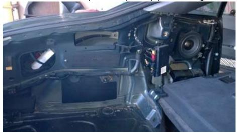
Driver Side Rear Speaker panel (Pull carefully or use pry bar as leverage to release the tabs)
