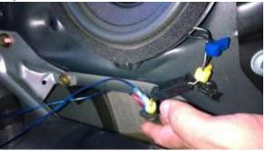
Run wires down Driver Side ¼ Panel to rear of vehicle.
