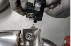
C) Rotate Scorpion valve so its in the same position as the O.E electronic valve motor.
