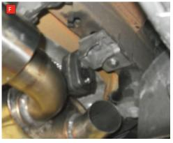
F) Before fitting the scorpion exhaust you need to adjust both of the rear mounting points. Remove the original mounting point retaining the original fittings. Using items 10,11 and 12 Bolt the bracket into the hole left by the original mounting point as shown in figure 'F'. Re-fit the original mounting point using the original bolt into the hank bush on the mounting bracket. This needs to be done for both mounting points either side of the rear silencer.
