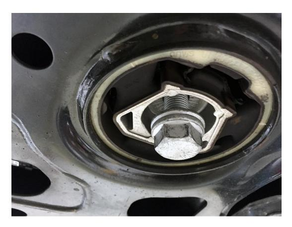
**Step 5** – With the factory bolt removed, you can install the Billet Aluminum Dobgone Mount Insert into the voids. It should be positioned with the 034 logo towards the front of the car.
