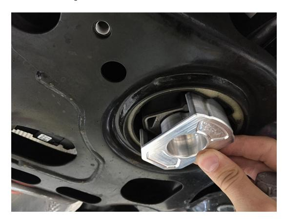
**Step 6** – Reinstall the factory dogbone mount bolt. Torque to 100 Nm.
