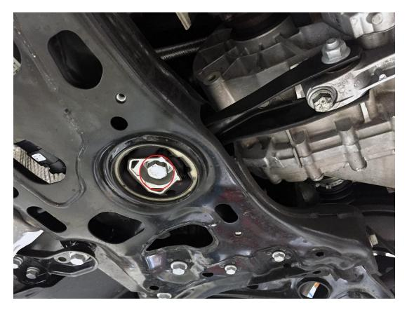
**Step 3** – Using the 21mm socket, remove the factory bolt.
