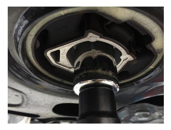
**Step 4** – Remove the bolt completely in order to install the 034Motorsport MQB Audi/Volkswagen Dogbone Mount Insert.
