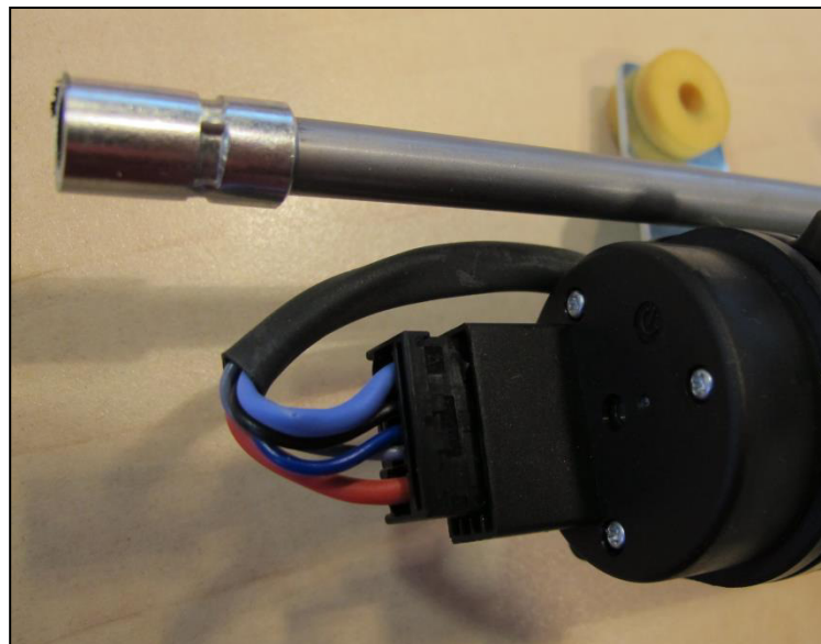
Fig. 5: Severed coupling sleeve at drive motor (for better clarity shown disassembled)
