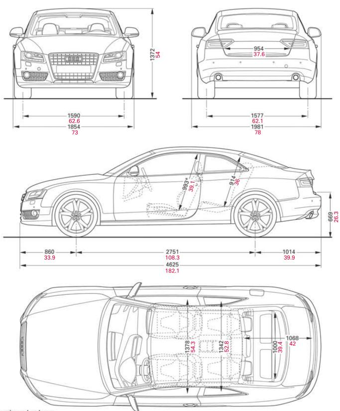
\* maximum headroom Dimensions in milimeters and inches Dimensions of vehicle unloaded
