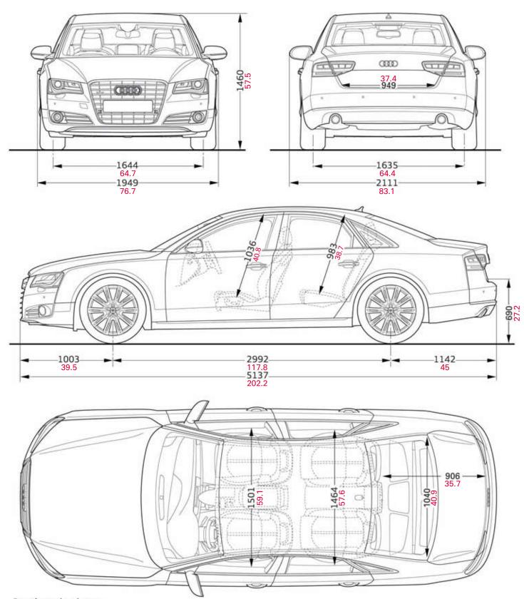
\* maximum headroom Dimensions in milimeters and inches Dimensions of vehicle unloaded
