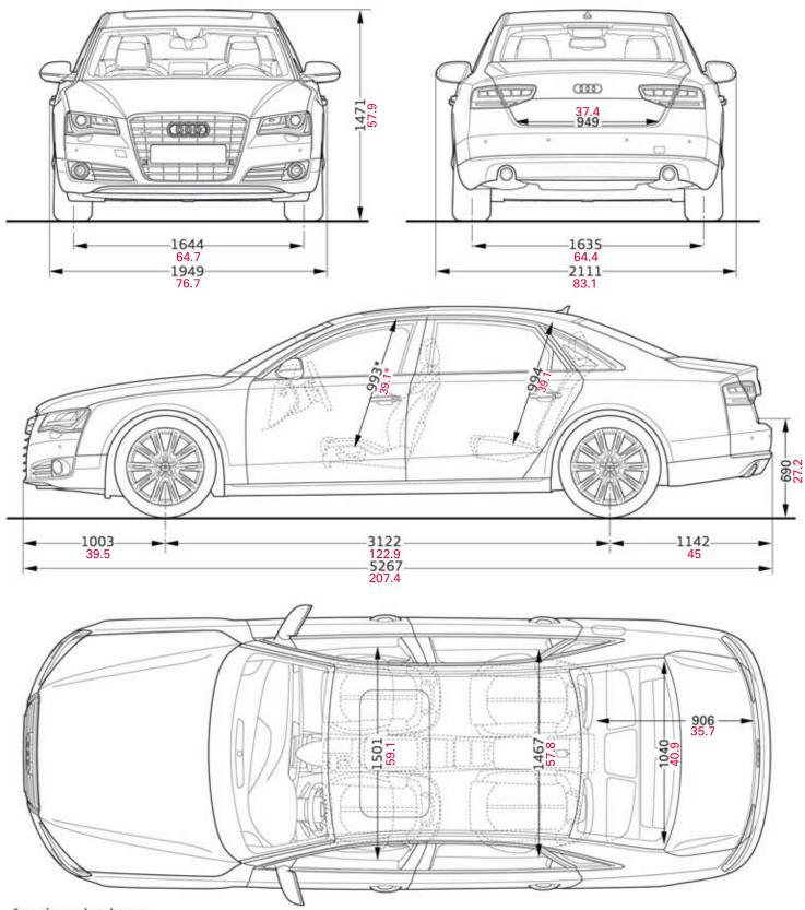
\* maximum headroom Dimensions in milimeters and inches Dimensions of vehicle unloaded
