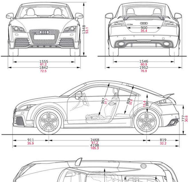
\* maximum headroom Dimensions in milimeters and inches Dimensions of vehicle unloaded
